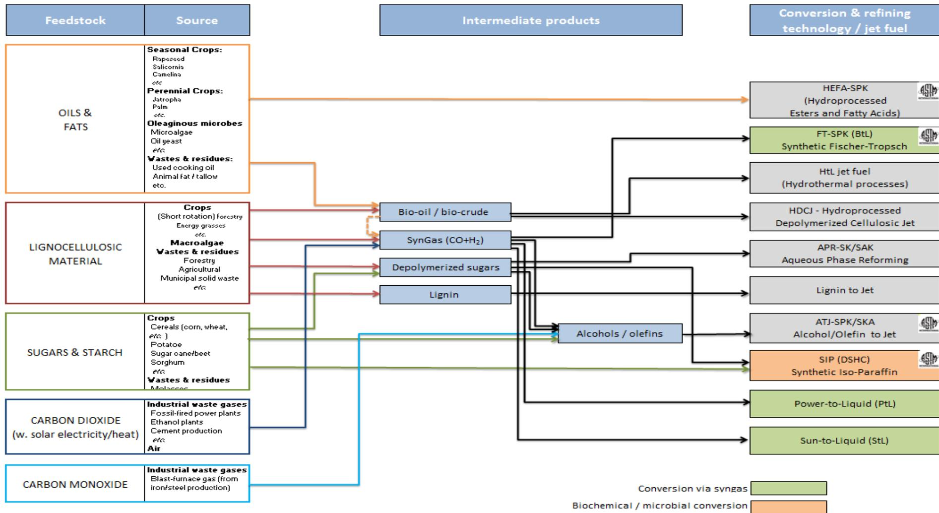
**Figure 1:** Schematic representation of the identified "landscape" of production pathways towards renewable jet fuel, defined by types of feedstock, conversion technologies and the feasible combinations thereof. Indication of ASTM certified pathways
