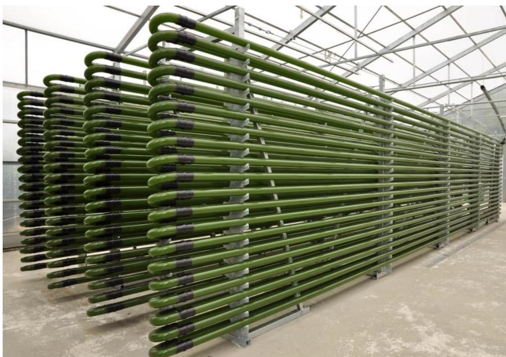
**Figure 4:** Photobioreactor (Wikipedia: ©IGV Biotech, CC BY-SA 3.0)
