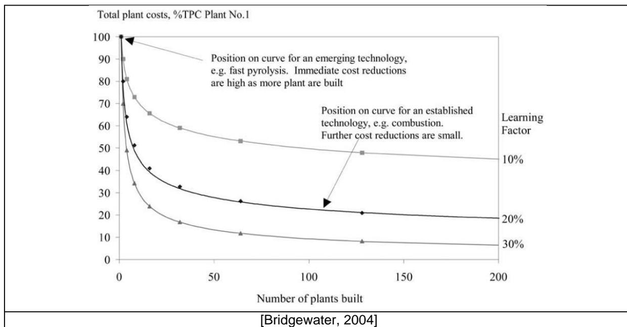
Figure 26: Industrial plant cost and learning factor v/s number of plant built
