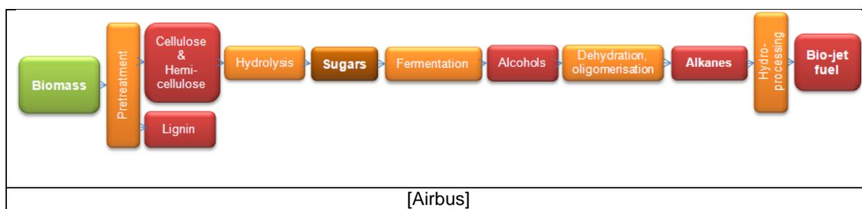
Figure 7: Detailed steps of Alcohol-to-Jet pathway
