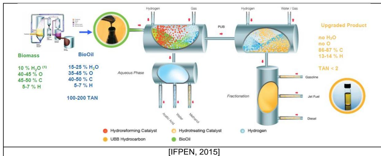
Figure 10: Typical Fast Pyrolysis with 2 steps upgrading of bio-oil to biofuels
