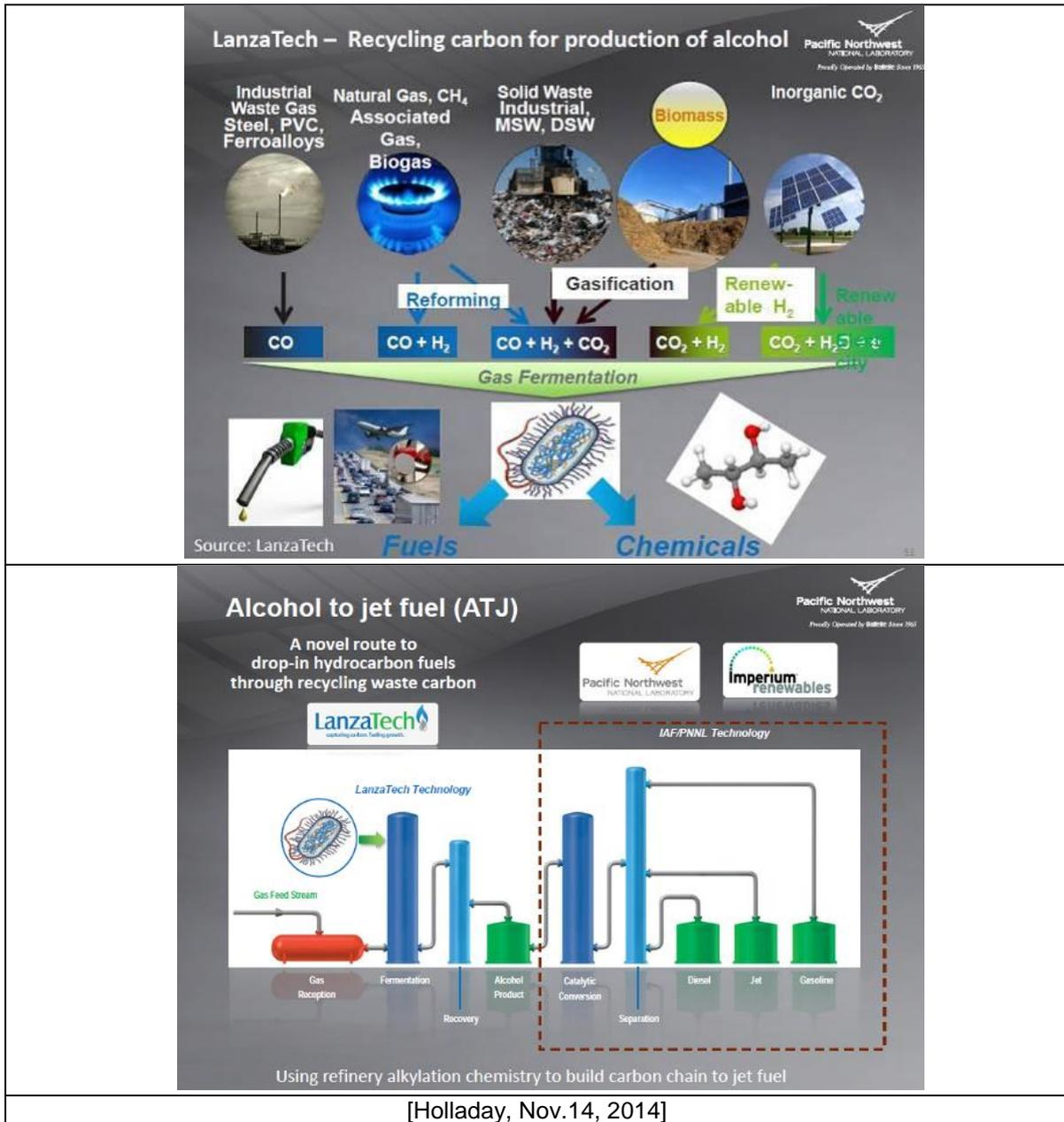
Figure 13: Lanzatech / Swedisch biofuels process from industrial gases process
