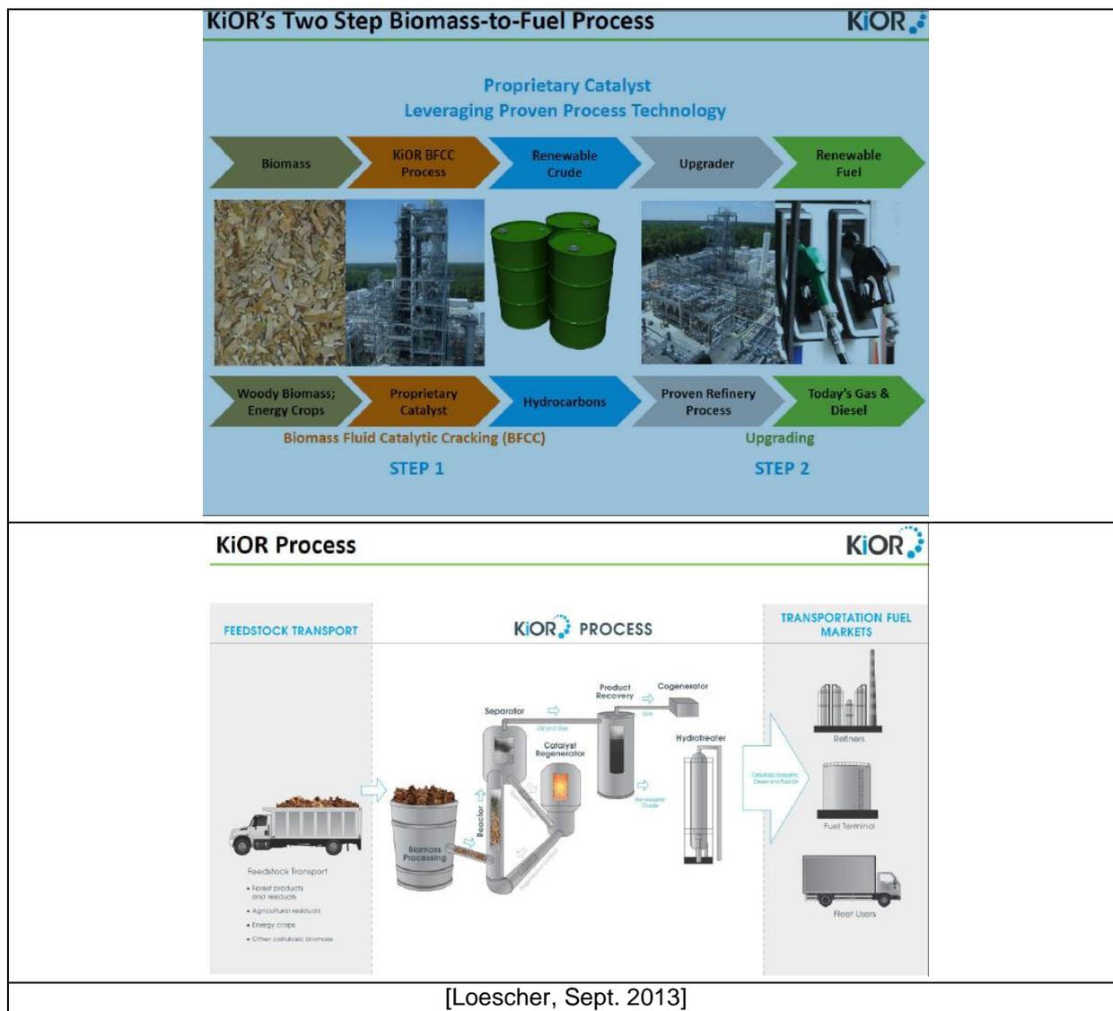
Figure 9: HDCJ/KiOR two-step process
