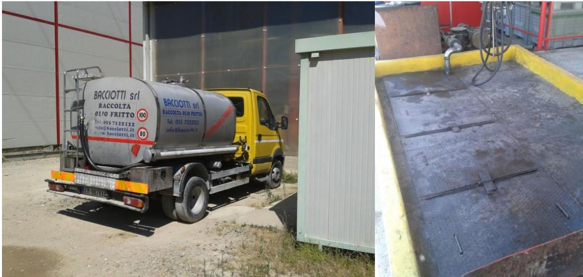
Figure 3: UCO collection by means of special vehicles that discharge the feedstock into a basement storage.
