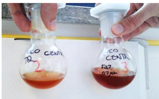
Figure 5: Used cooking oil samples: pure and filtered at 0.7  $\mu\text{m}$  (according to UNI EN 12662).
