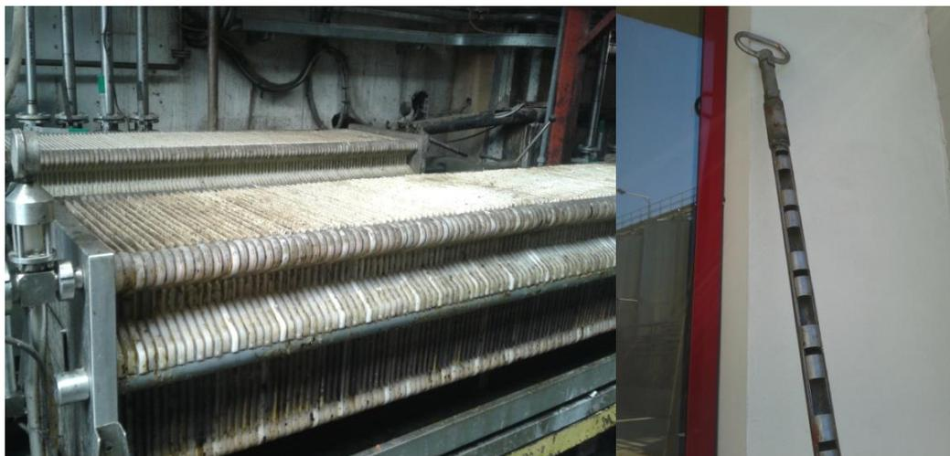
Figure 4: SILO Industrial filtration and the special probe (Sonda Marsigliese) for oil sampling.
