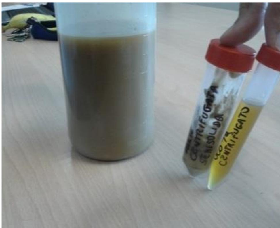
Figure 2: On the left side, raw UCO. On the right side, the residual of centrifugation (left) and the separated oil (right).
